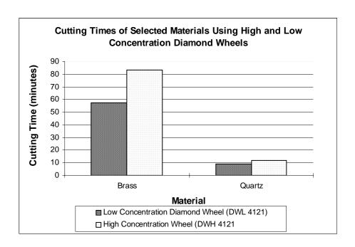
Chart illustrating the variation in cutting time as a function of diamond wheel concentration. As can be seen in the graph above, the cutting time is much lower for low concentration diamond wheels as compared with high concentration wheels. The effect is greatest when cutting ductile, metallic materials as compared to ceramic materials.
